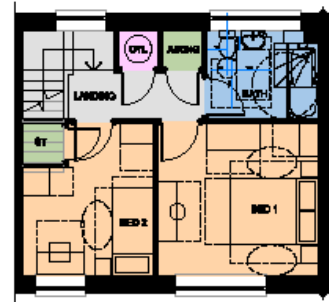
FIRST FLOOR LAYOUT HOUSE TYPE A 3 BED / 2 BATH HOUSE Frd Floor Area = 20.3sq²
